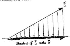
$B\cos\theta$  is the projection of  $\vec{B}$  along the direction of  $\vec{A}$ . (You can think of  $\vec{A}$  as the ground. Then, with the sun directly overhead,  $B\cos\theta$  is the signed-length of the shadow. You get a positive-sign if the shadow's arrow points in the same direction as  $\vec{A}$ . You get a negative-sign for the opposite direction.)
